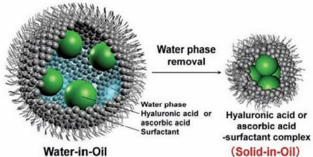
Fig. 1 Schematic illustration of solid-in-oil compared with water-in-oil.
